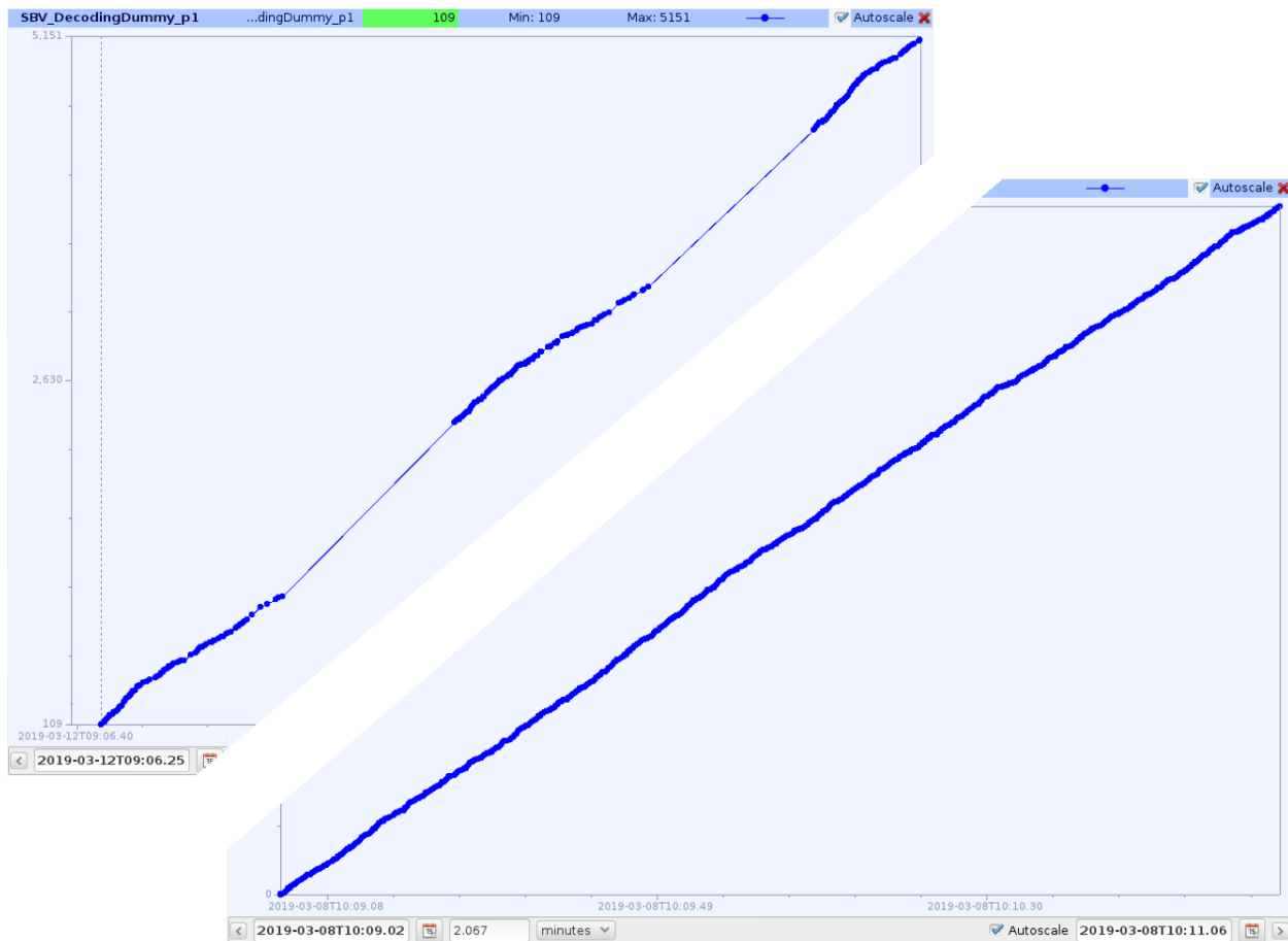
Fig. 10 Current test results for deferred parameter value playback in EGS-CC, showing a live UDD on the left and a playback UDD on the right.
